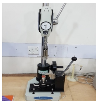
Figure 23 Button pull tester
