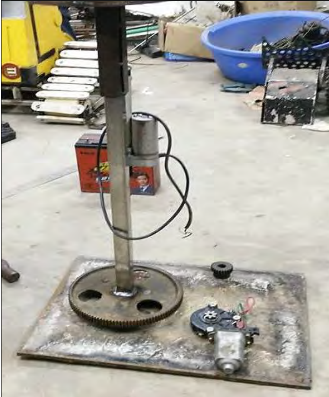
Figure 5.3-1 The main base of the body without wheels and box cover
