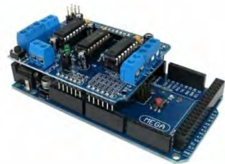
Fig 9. Motor Shield placed on Arduino MEGA
