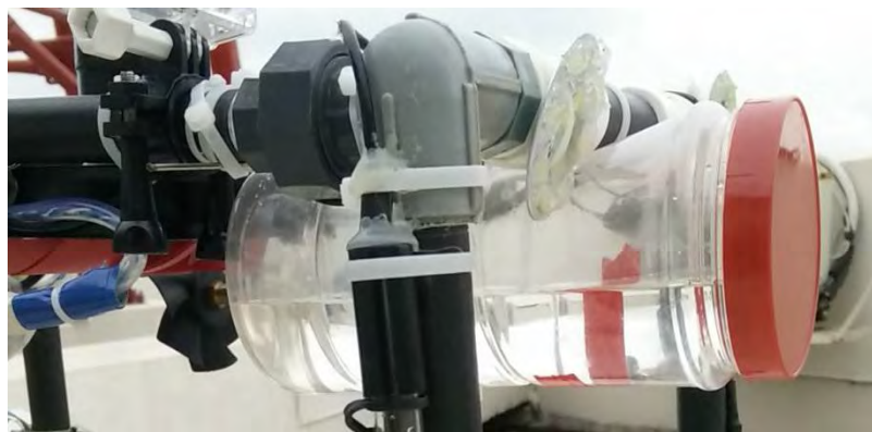
Fig 16. Attached container for Buoyancy management.
