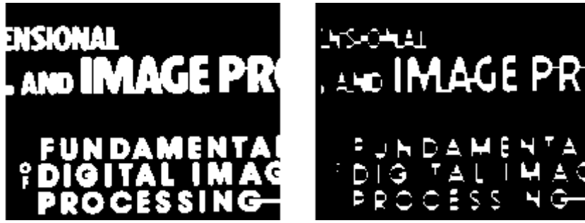
Fig 3.7 Binary Image and Hit and miss transform of an elongated 2 \times 5 structuring element
