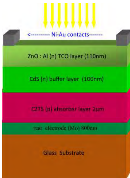
Fig-1:A typical schematics representation of CZTS, CdS solar cell is shown in fig: 1.
