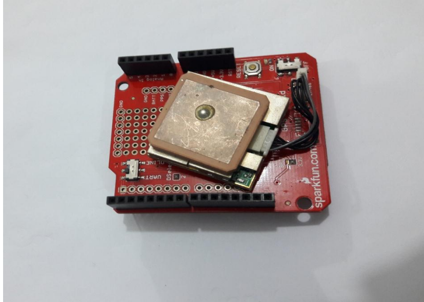
Fig 13: Elements soldered together with EM-506 antenna attached through connector wire
