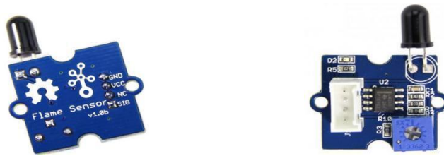
Figure-3.7 Top and Bottom View of Grove Flame Sensor
