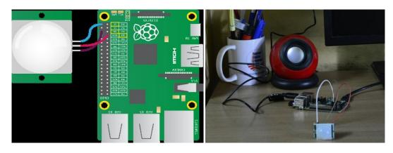
Fig. 15b: Connection between PIR and Pi
