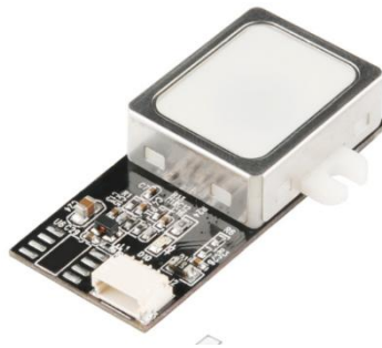
Figure 3.2.2: Fingerprint Scanner- TTL (GT-511C3)
