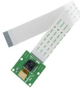
Figure 3.2.13: Raspberry Pi camera module
