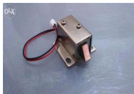
Figure 3.2.9: Electric Solenoid Mini Door Lock DC 12V
