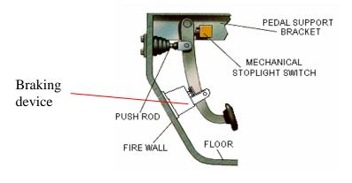
Fig 7: Side view of the brake pedal
