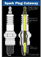
Fig 3: The spark plug
