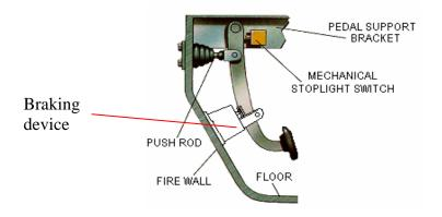
Fig 15: Mounting of the braking device
