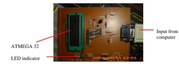
Fig 11: The downloader Circuit
