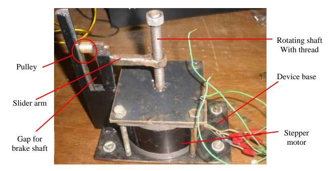
Fig 14: Braking Device
