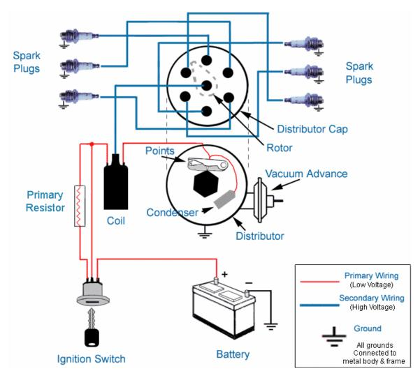
Fig 5: The Ignition System Diagram
