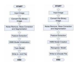
Figure 1: Flow chart of training and recognition procedure
