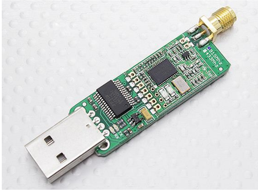
Figure 3.12 Telemetry Radio (Ground Station unit)
