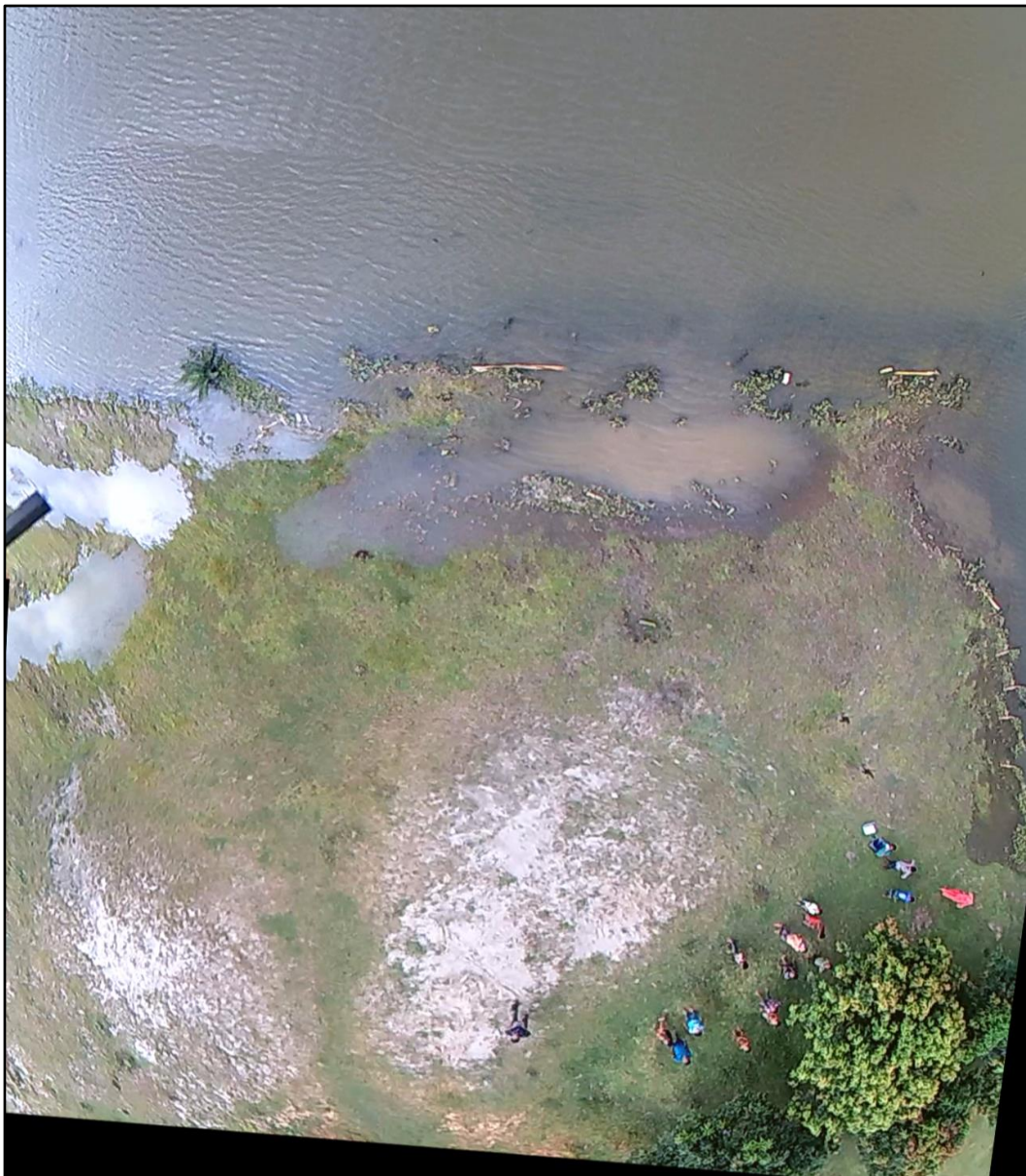
Figure 6.2: Digital mosaic of two consecutive image frames after necessary correction and geo-referencing operation. The relatively rough water surface with certain textural pattern is readily visible in the image areas corresponding to water area.
