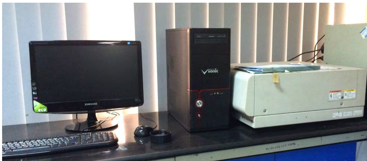
Figure 2.2: Picture showing UV-Visible spectrophotometer
