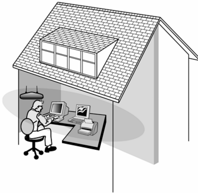
Fig – 6.7 Minimized leakage inside a residence.
