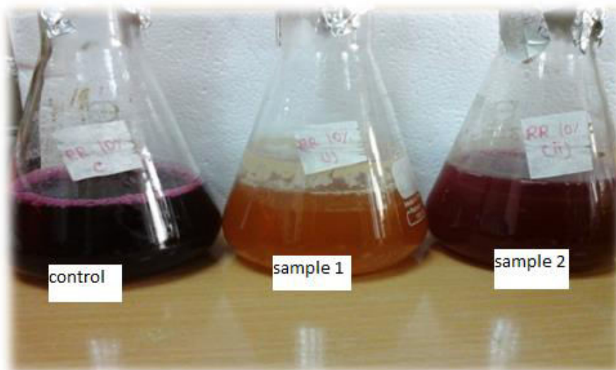
Figure 14: Reactive Red 10% samples. Here middle conical flask's dye containing media's color is degraded. (left conical flask = Control, middle conical flask sample 1, right conical flask = sample 2)
