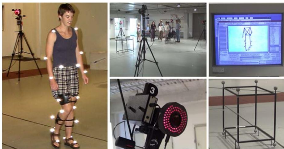
Fig.3.11. Gait laboratory of The University of Auckland (in 2000). Left: walking subject with markers. Middle: walking area (top) and one of the fast cameras (bottom). Right: generated animated 3D stick figure (to) and camera calibration unit (bottom).
