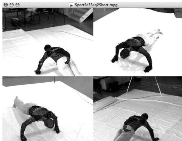
Fig.3.14. Human poses are tracked using a generic 3D model of the upper human body; the figure shows the backprojection of the recorded 3D motion into the original 4camera image sequence, also demonstrating model movements of occluded body parts
