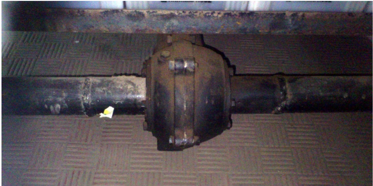
Figure 4.2.1: The differential at the rear of the solar car.
