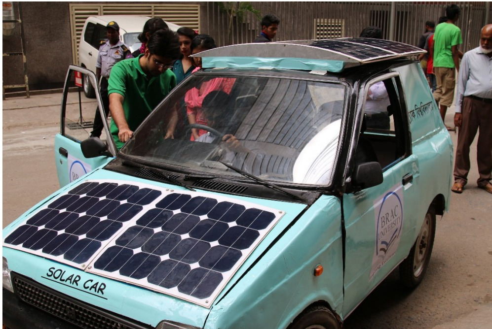
Car with solar panels placed on the roof and bonnet
