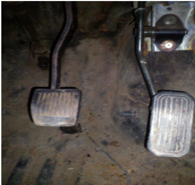
Figure 4.3.1: The accelerator pedal (on the right) with the brake pedal (on the left).
