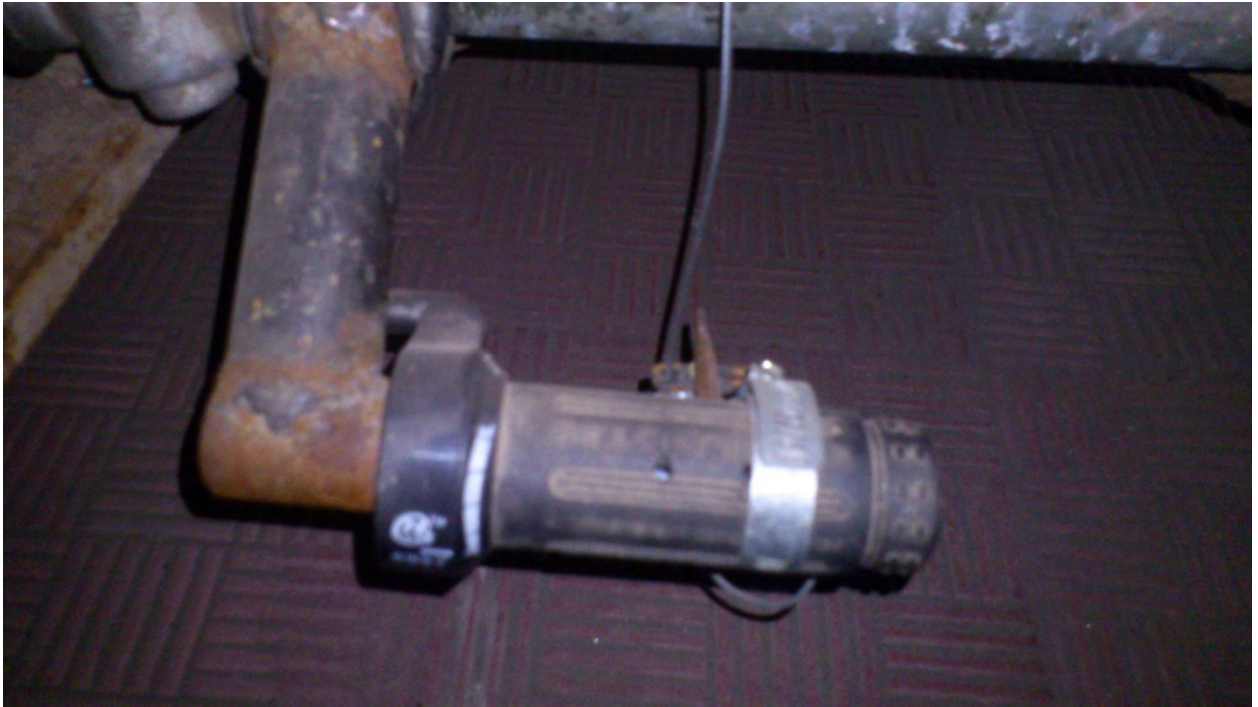
Figure 4.3.1: Hand throttle connected to the pedal accelerator via a cable.
