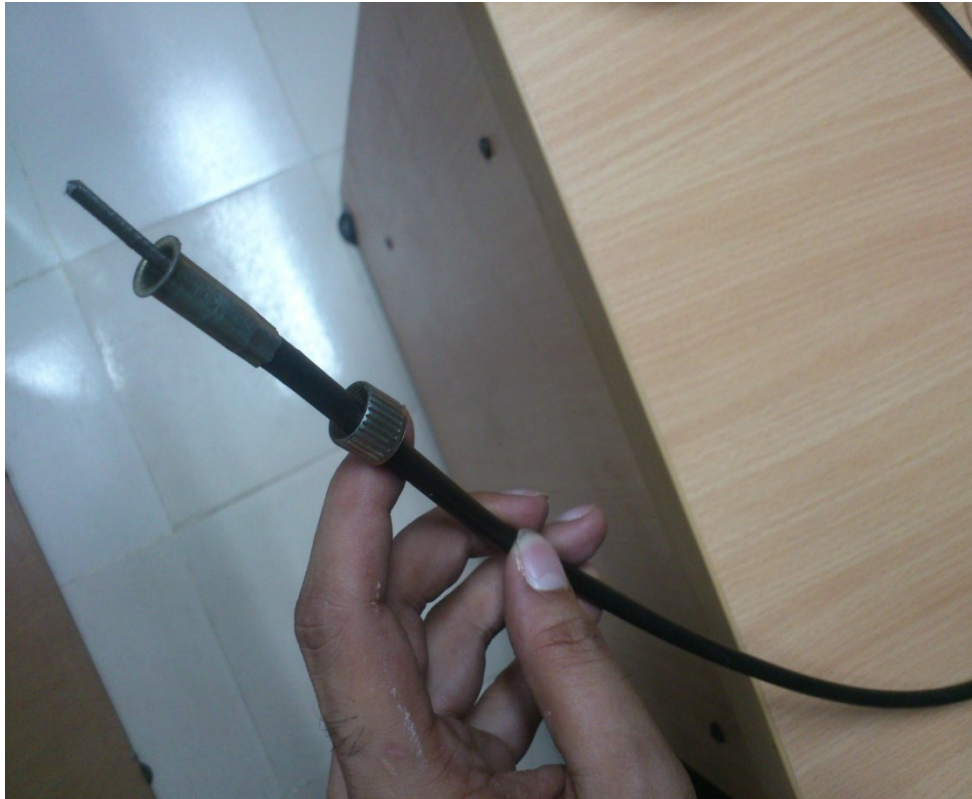
Figure: Cable with a moveable wire inside.
