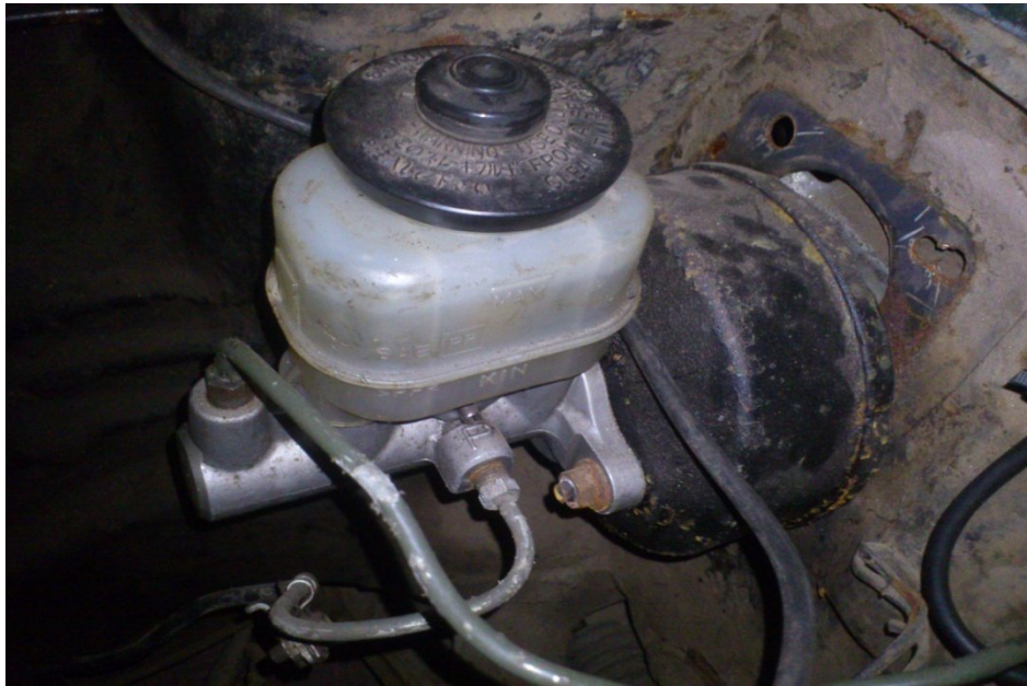
Figure 4.1.2.2 (b): Master cylinder used in the solar car.
