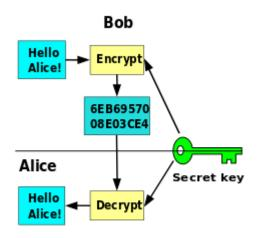
*Figure 4.11:* **Symmetric-Key Cryptography** A single key is used for both encryption and decryption.
