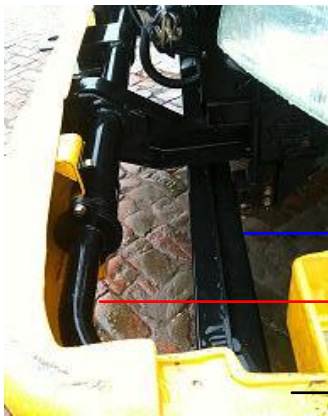
Steel made bumper with crash guards
