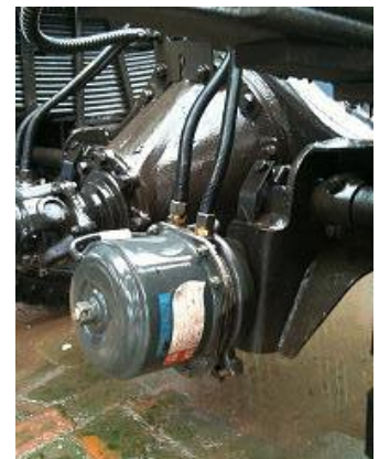
Large air brake actuator (TVS) for highest brake performance
