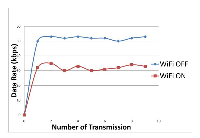
Fig10 : Data rates in presence of Wi-Fi interference
