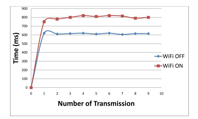
Fig11 : Time Taken in presence of Wi-Fi interference
