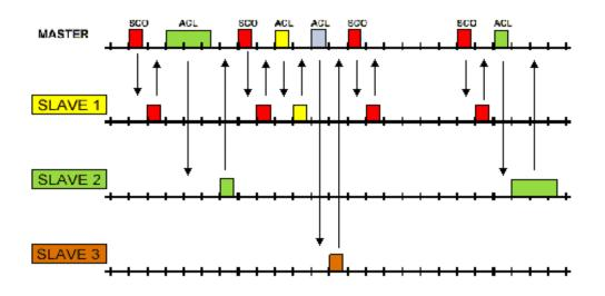
Fig 2:- Master and slave operation
