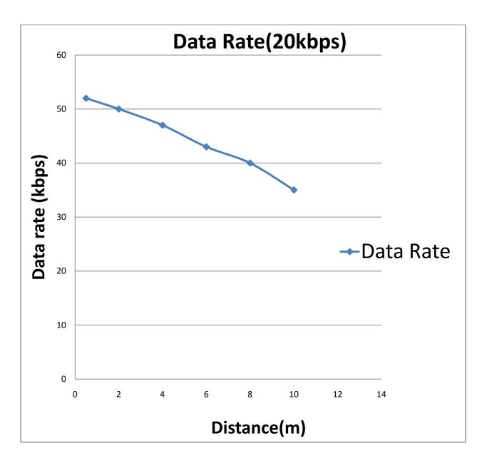
Fig8 : Data rate Vs. Distance
