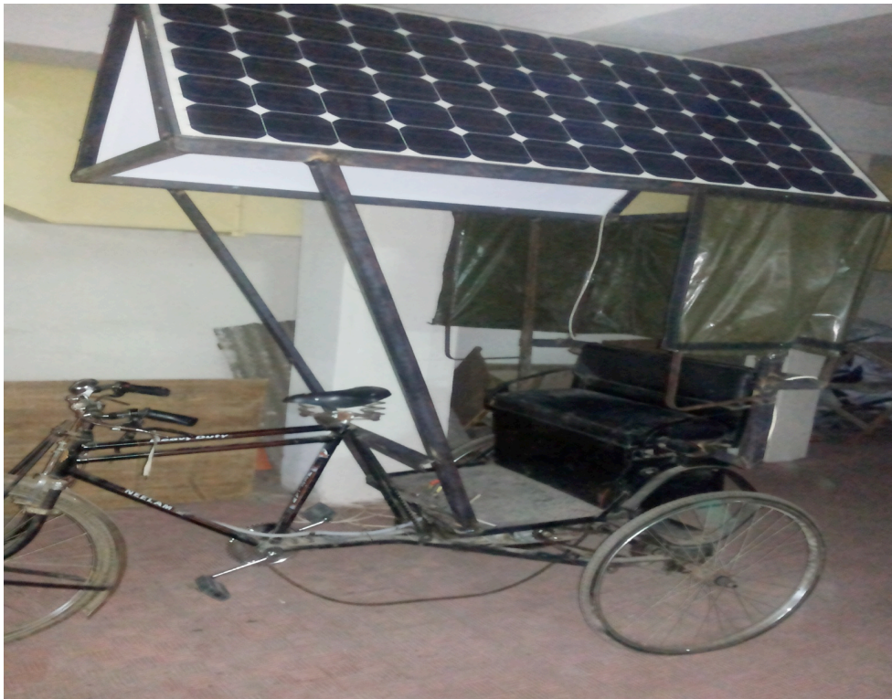
FIG. 5.7 INCLINED PANEL STRUCTURE
