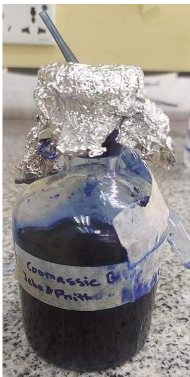
Figure 3.10: Coomassie Blue dye prepared to stain the biofilms using CBB G-250 powder
