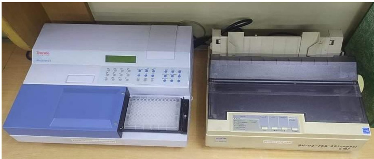
Figure 3.13: MultiscanEX ELISA Machine by Thermo Scientific
