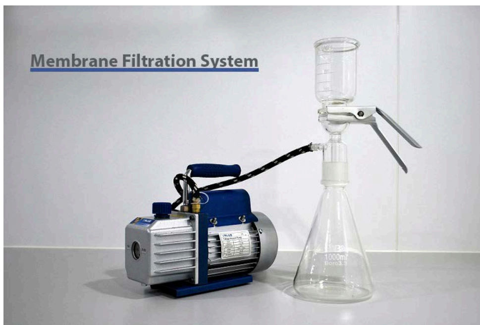
Figure 2.4.1: Membrane Filtration System
