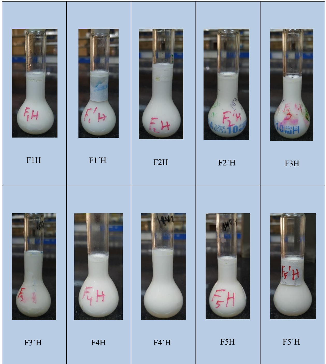
Figure 4 : Dilution test with 0.1N HCl
