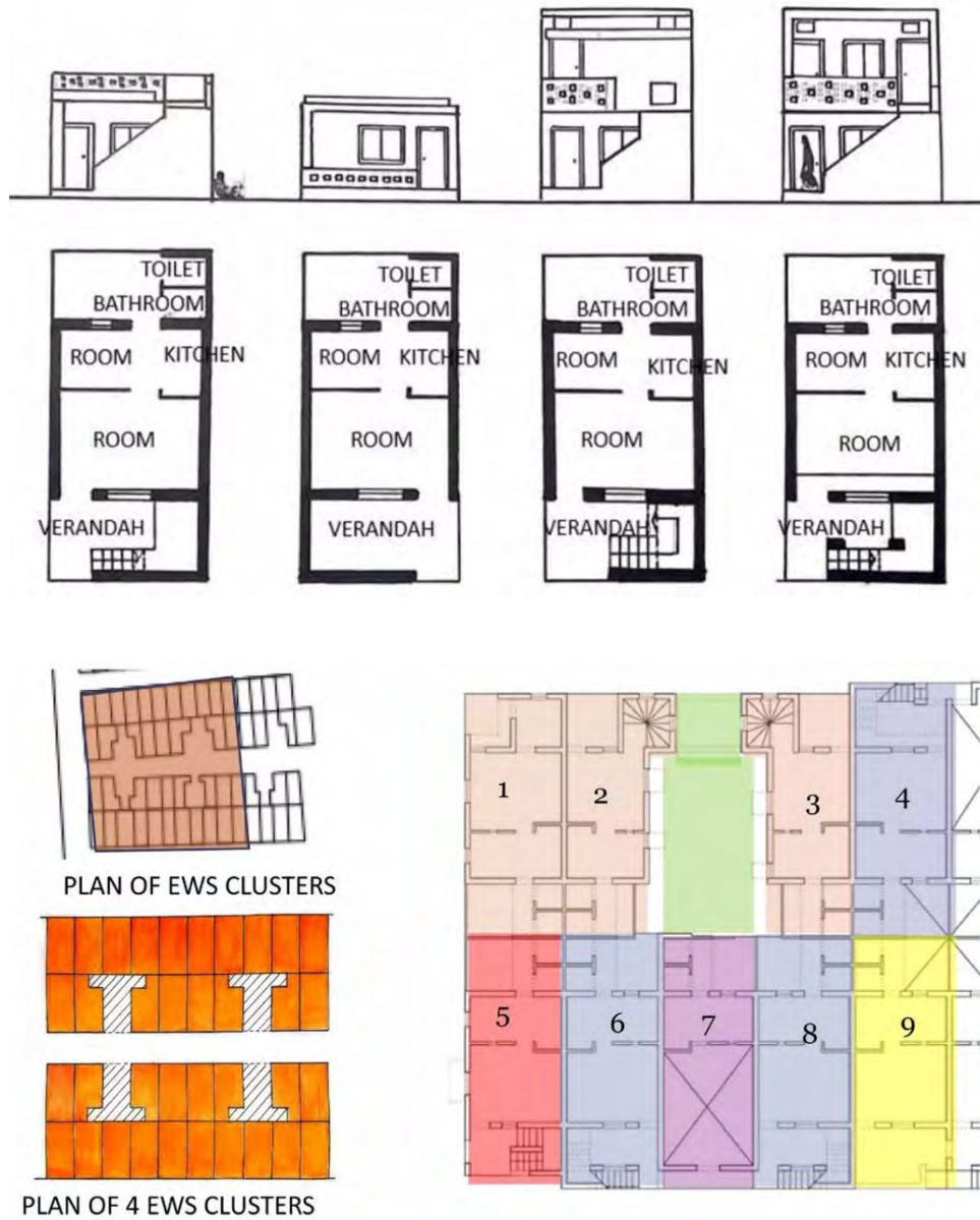
Figure 4.2.4: Figure showing the plans of the housing typology for EWS group. Source: (Ahmed, 2018)
