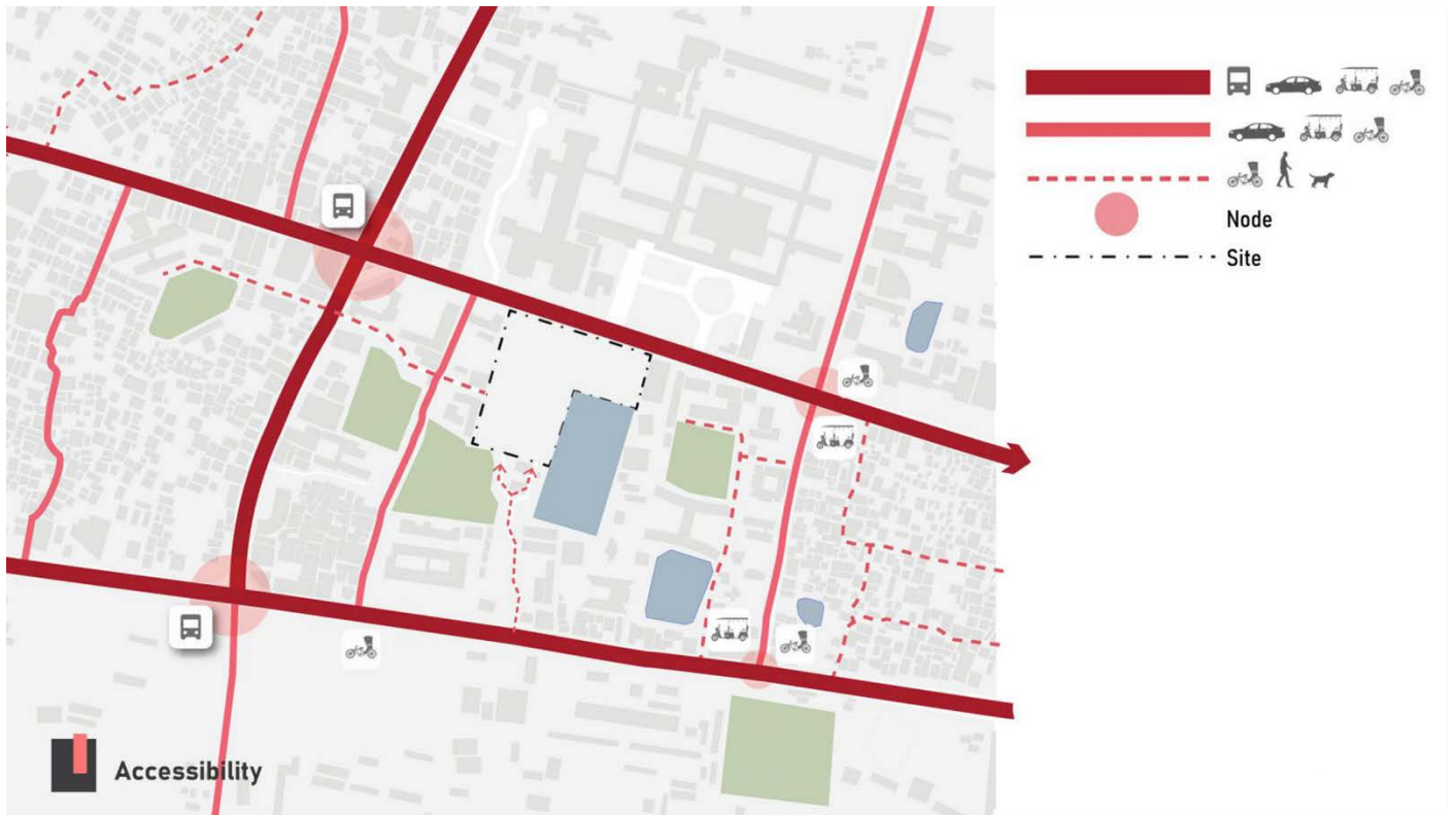
fig 12: Road Typology and Accessibility around the site. Source: Author
