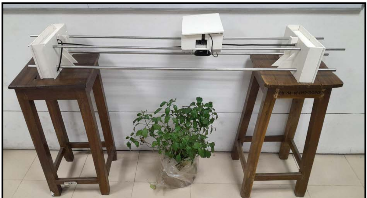
Figure 24: Prototype of our disease detection system on top of the timing belt device.
