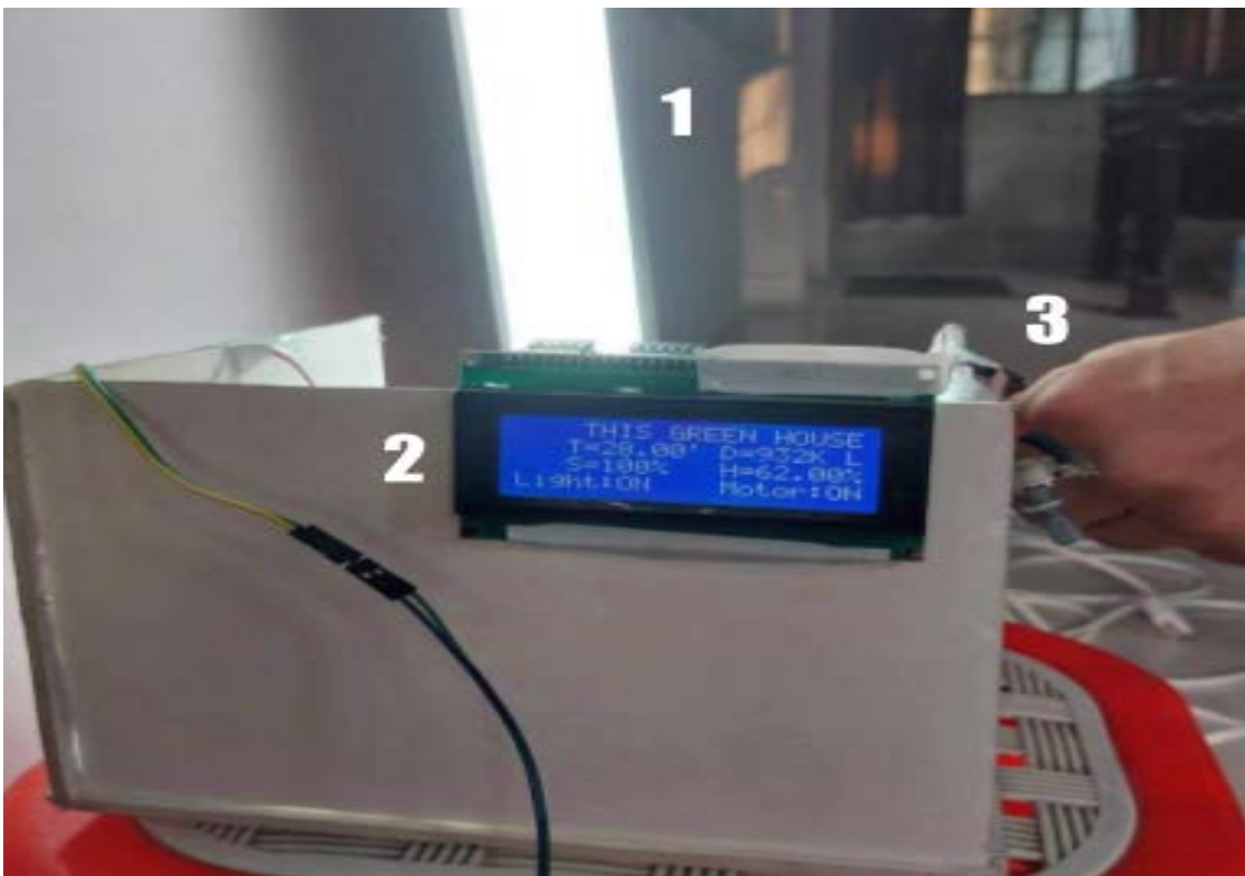
Figure 36 : Sensing the light intensity of the environment and External Light gets on (1.External Light 2.Notification panel 3.LDR sensor )
