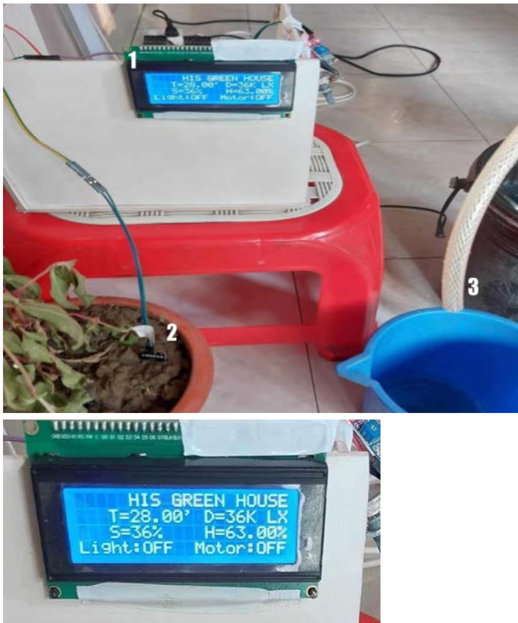
Figure 34: Sensing the dryness of the soil and water motor gets off (1.Notification panel 2.Soil Moisture sensor. 3. Water Motor )
