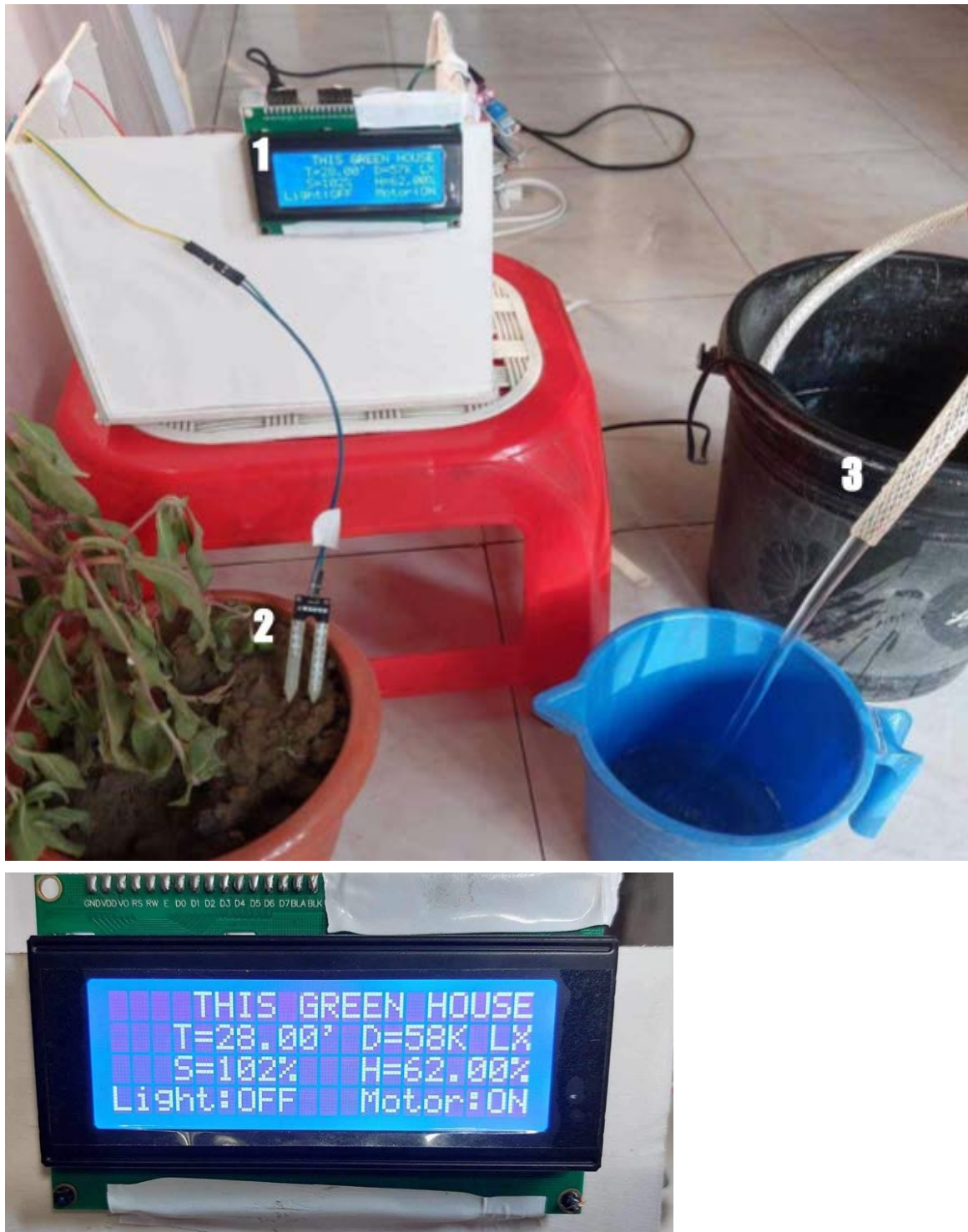
Figure 33: Sensing the dryness of the soil and water motor getting on (1.Notification panel 2.Soil Moisture sensor. 3.Water Motor )
