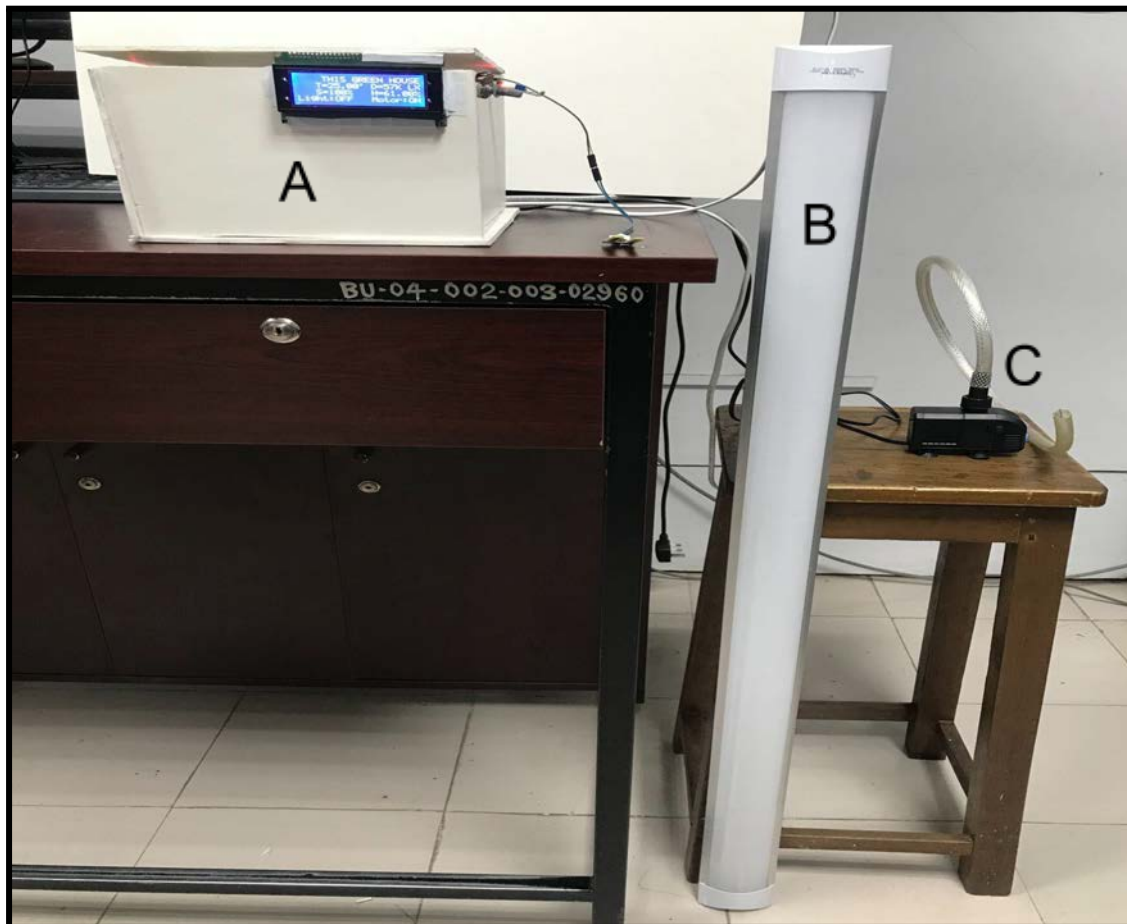
Figure 28: (A) Complete Environmental Notifications and Monitoring Control System with Notification Panels. (B) Additional 40W LED Light & (C) Submersible Water Pump.
