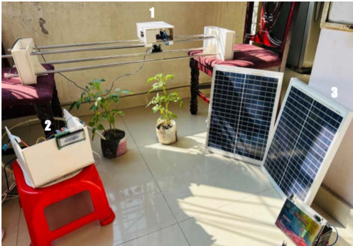
Figure 37: Hardware prototype of the completed project (1. Disease detection 2. Environmental monitoring 3. Solar system).
