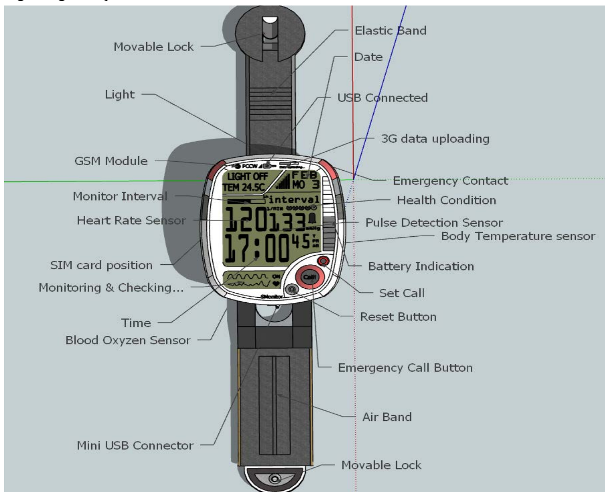
Fig 5: 3D design of Oxy-Cardio Band
