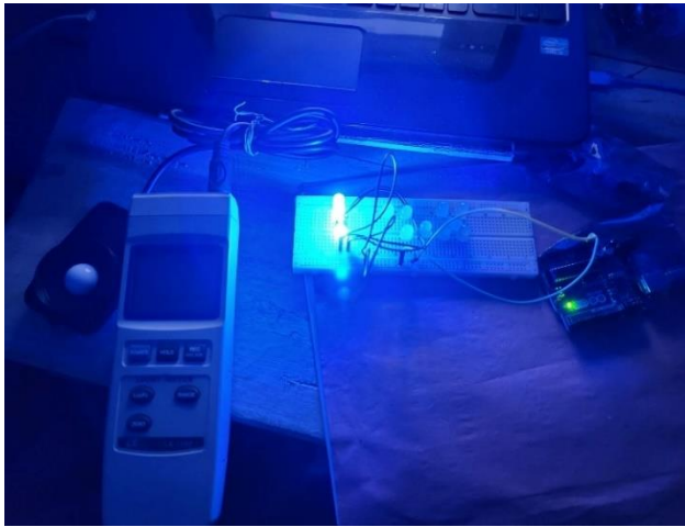
Figure 15: Measuring intensity of Blue LED in LUX meter
