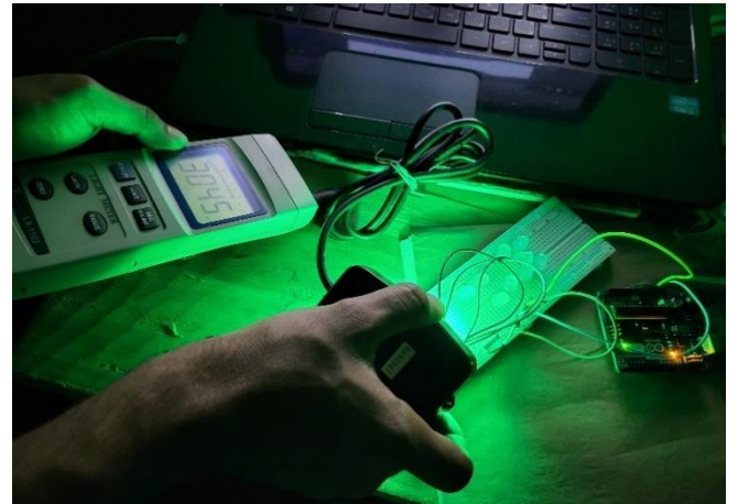
Figure 16: Measuring intensity of Green LED in LUX meter
