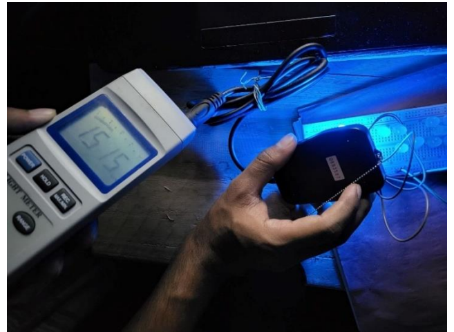
Figure 15: Measuring intensity of Blue LED in LUX meter
