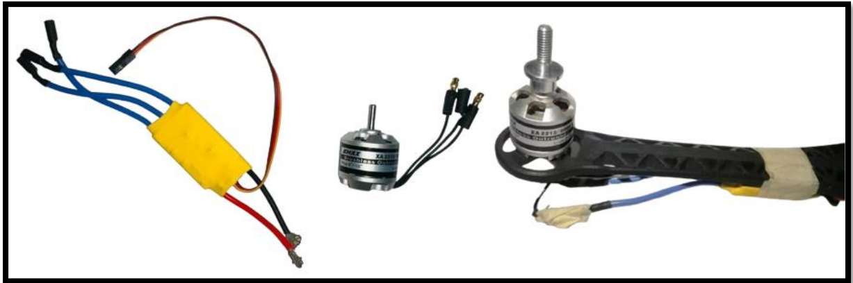
Fig.24. Mounting motors and ESCs.
