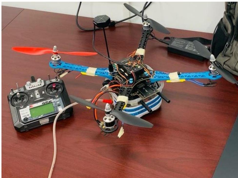
Fig.36. Prototype of design approach 1 unmanned aerial vehicle (UAV) based water sampler.
