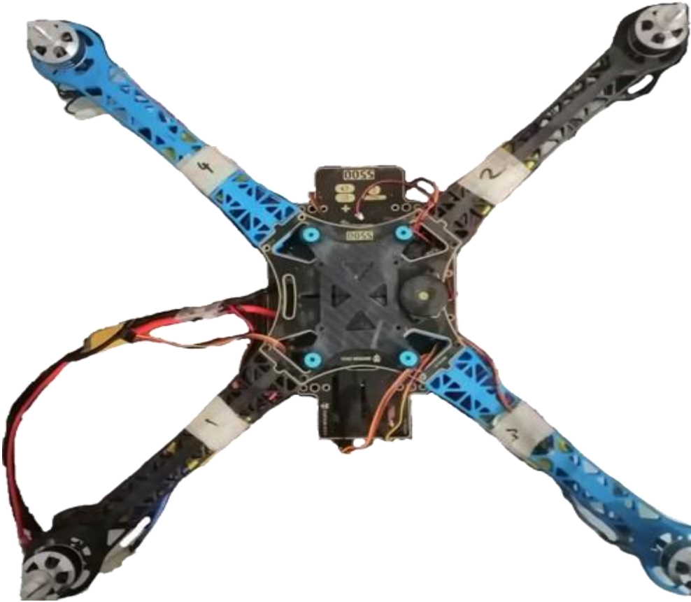
Fig.26. Addition of buzzer and shock absorber.
