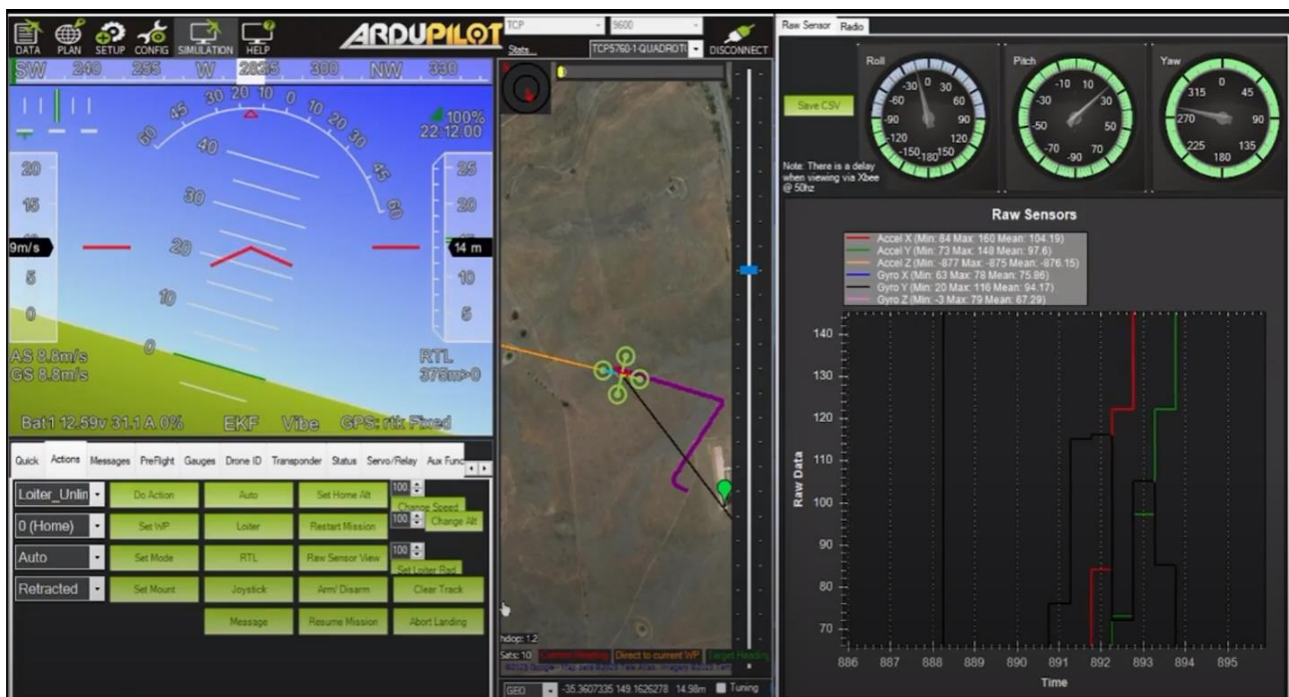
Fig.14. ArduPilot flight simulation for design approach 1.
