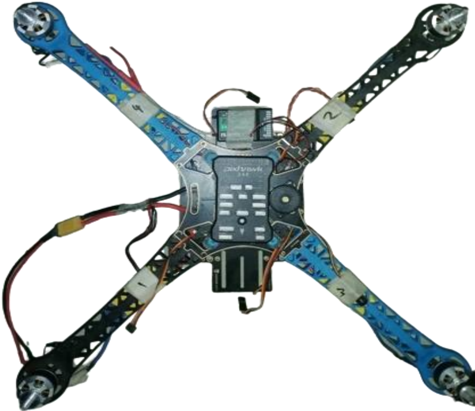
Fig.27. Addition of Pixhawk and RC receiver.
