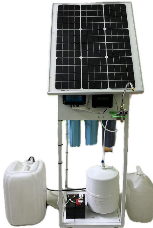
Fig 5.3: Final prototype design
