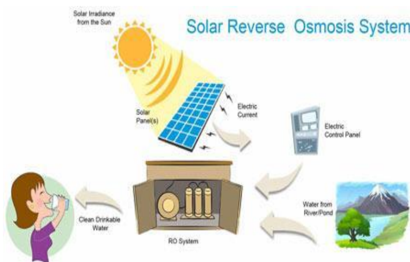
Fig 2.1: A solar powered water purifier using reverse osmosis [20]
