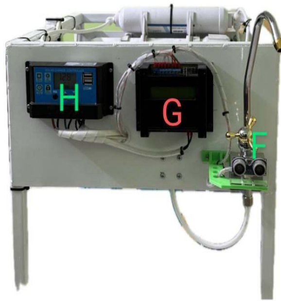
Fig 5.5: Final prototype design, charge controller and sensor module
