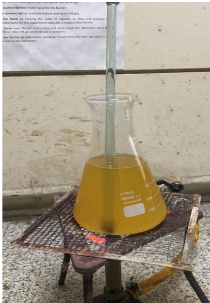
Figure 2.2: Nutrient agar and distilled water was boiled in a conical flask
