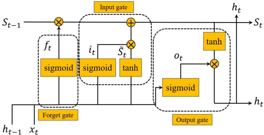
Figure 2.1: Structure of a LSTM memory block
