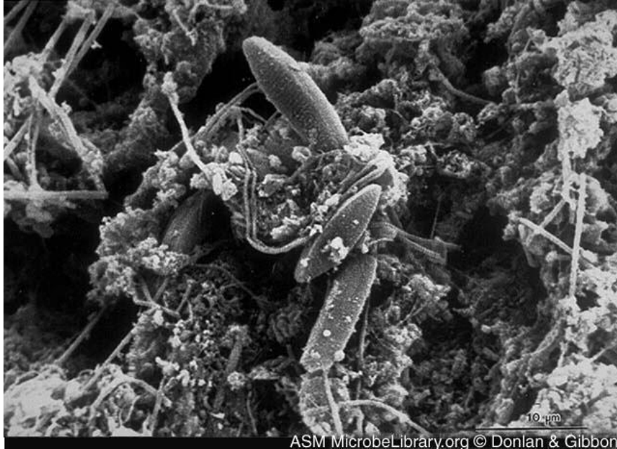
Figure 1: Scanning electron micrograph of a native biofilm that developed on a mild steel surface in an 8-week period in an industrial water system.
