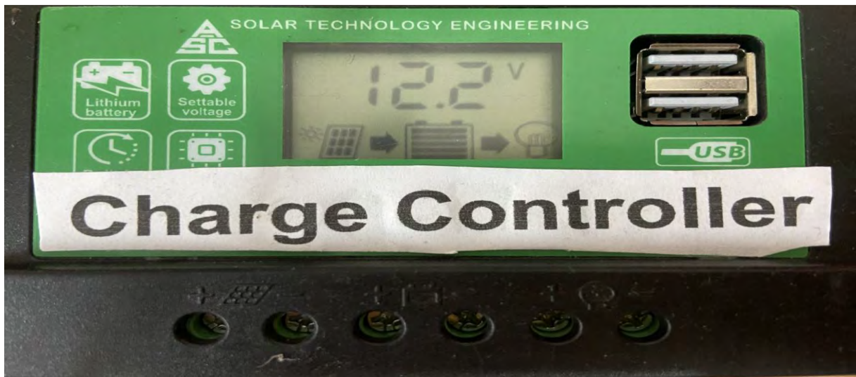
Fig 5.9: Charge controller (keep the battery safe from overcharging)
