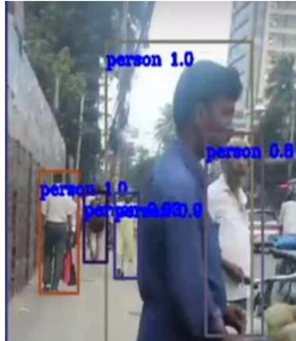
Figure 4.13: Detecting Object with bounding box with class
