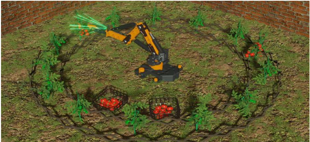
Fig. 4.2.19. Science box locating vegetables using 3D coordinates and laser sensors
