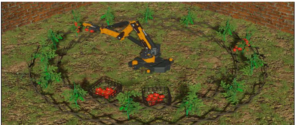
Fig. 4.2.20. Science box harvesting ripe vegetables using picture segmentation
