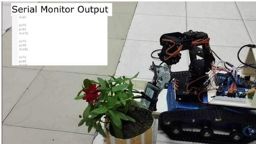
Fig 5.3.11- NPK sensor and Serial Monitor
