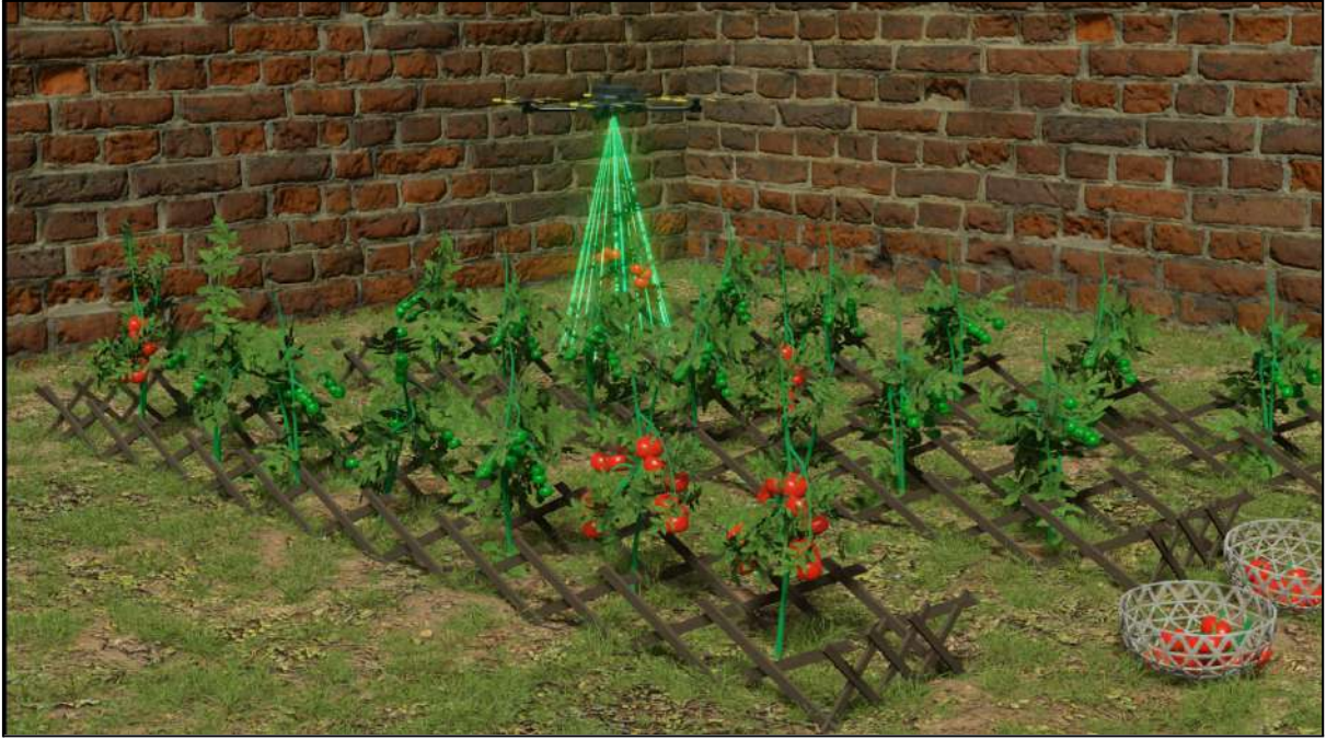
Fig. 4.2.11. UAV locating vegetables using three-dimensional coordinates and laser sensors
