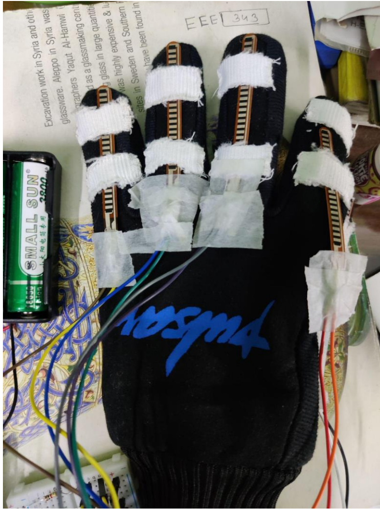
Figure 5.5 Placing flexi sensors on the unaffected hand glove
