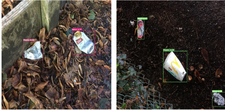
Figure 5.9: Predicted wastes after training the YOLOv7 model
