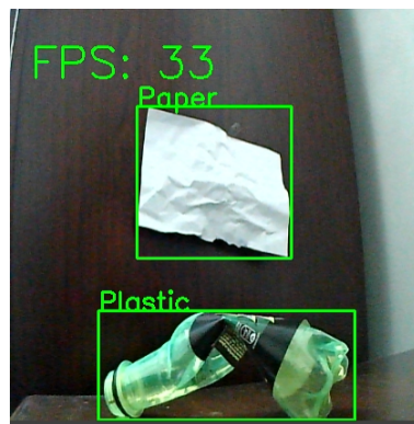
Figure 5.10: Real-time waste detection from video with webcam
