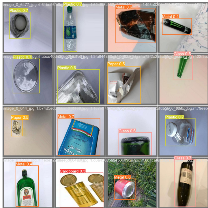
Figure 5.11: Predicted wastes after training YOLOv5x model
