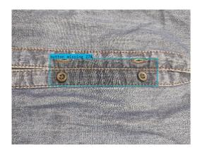
Figure 5.4: "missing button" class test image result
