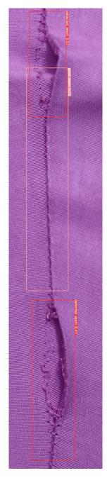
Figure 5.9: "good seam" class test image result after 100 epochs
