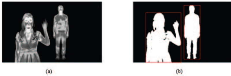
Figure 2.4: Hot-spot algorithm - (a) the original image and (b) binary with humans detected
