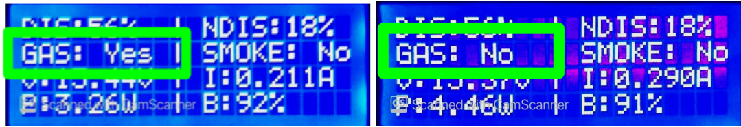
Fig. 64. Gas is detected
