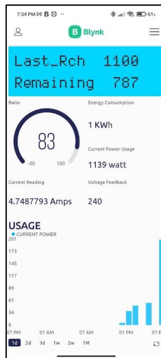
Fig 30: The User Interface we designed using the Blynk App
