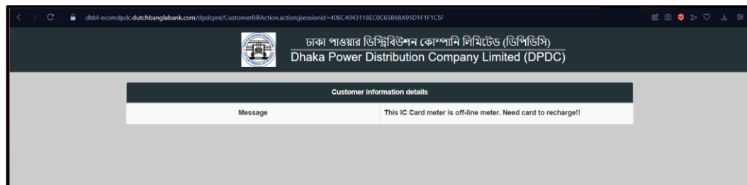
Fig 04: DPDC web (Customer information for offline meters).
