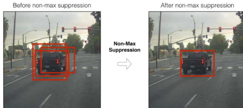
Figure 5.7: Before and After of Non-max suppression[11]
