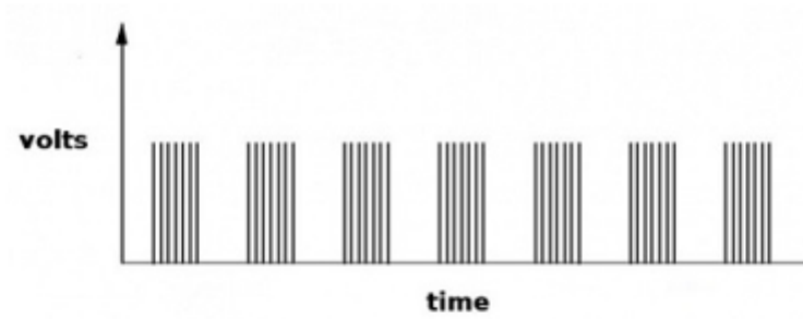
Fig: At frequency of 38kHz each pulse is turned on and off
