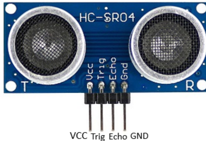
Figure 3.2: Ultrasonic Sensor that has been used for obstacle detection
