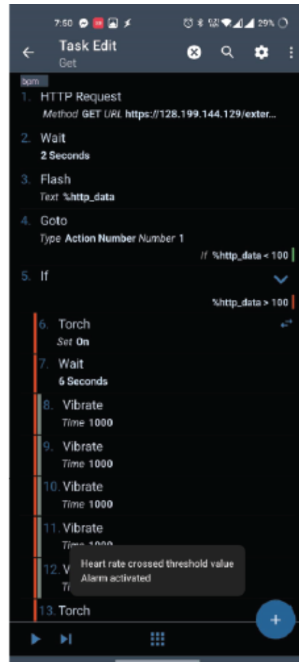
Fig 3.12: Alarm activation condition
