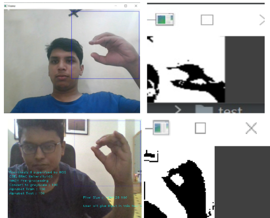
Figure 9.3: Gesture of alphabet “C” and “O” which look quite similar in grayscale form
