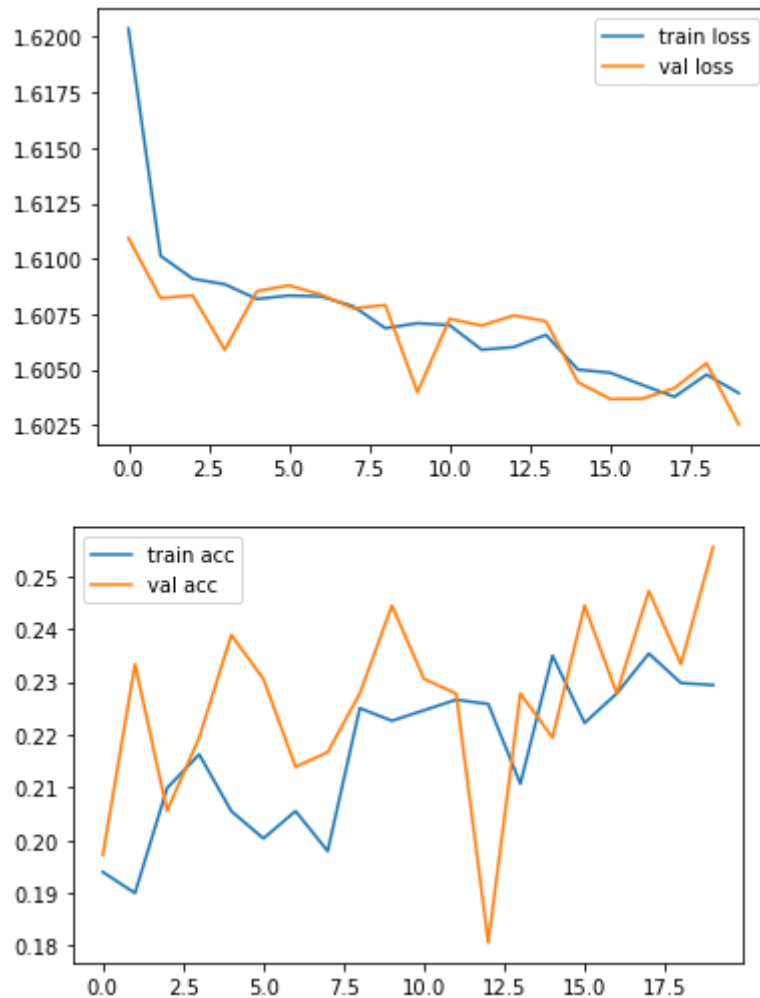
Figure 5.27: MobileNetV3 Large Loss-Accuracy Curve (Lowered)
