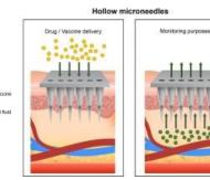
2017). Much research is now being conducted on the use of microneedles to encapsulate antigens in polymeric particles. Particle-based vaccines are frequently administered by hollow microneedles (Chu et al., 2019). The vaccination antigen is put into hollow needles, which are then inserted into the skin, where the vaccine antigens are dispensed (Niyomtham et al., 2017). An automated syringe containing microneedles that control the flow of antigen-containing gel inside
