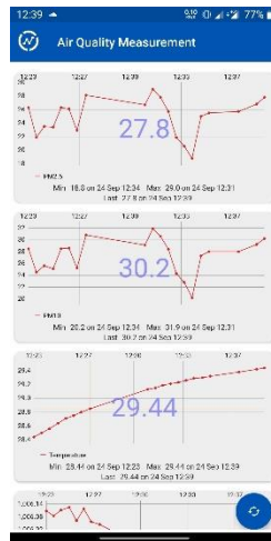
Figure 3.19: Presentation of values in the IoT platform ThinSpeak using an android application
